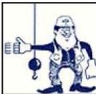
**RAISE THE BOOM AND LOWER THE LOAD:** With arm extended, thumb pointing up, flex fingers in and out as long as load movement is desired.
